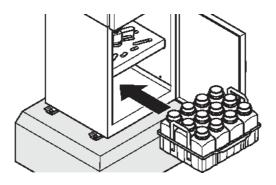
Fig. 26: Put the empty bottles in the housing
