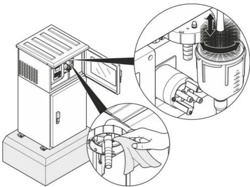
Fig. 40: Clean the dosing vessel
