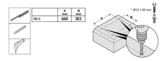
Fig. 5: Prepare place of installation
