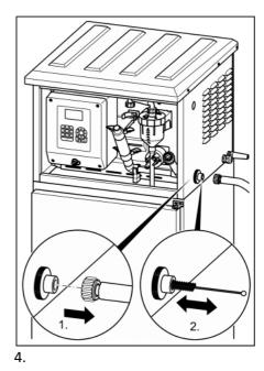
Fig. 42, 1-4: Cleaning measuring tube (flow-proportional dosing-system)
