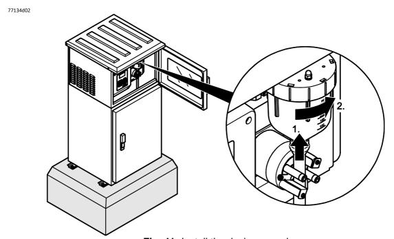
Fig. 41: Install the dosing vessel
