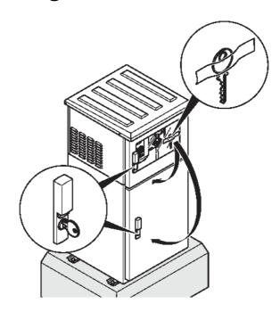
Fig. 13: Storage location of key (only with option "Key")
