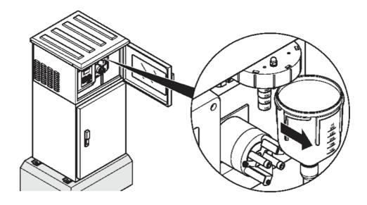
Fig. 20: Remove the plastic dosing vessel
