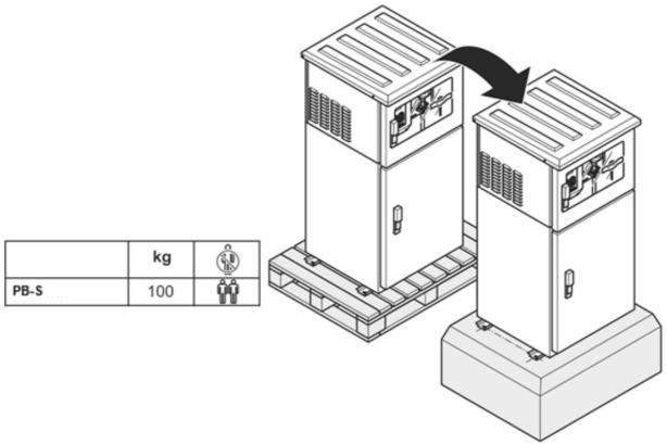
Fig. 7: Set up the equipment
