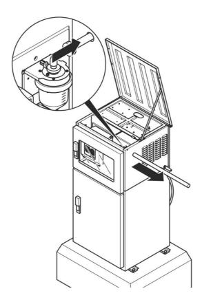
Fig. 14: Feed the suction hose through housing opening
