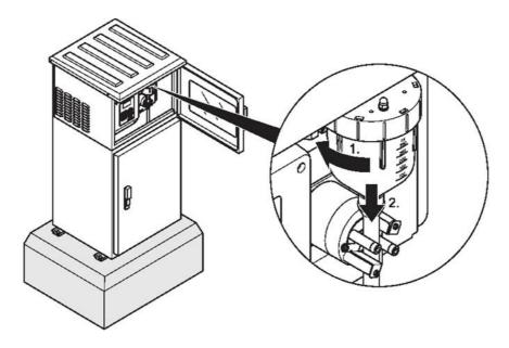
Fig. 38: Release the dosing vessel
