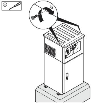
Fig. 17: Screw down the lid tightly
