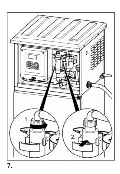
Fig. 43, 5-7: Cleaning measuring tube (flow-proportional dosing-system)
