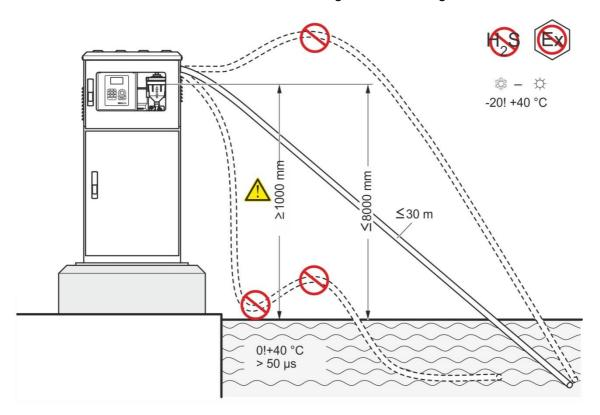
Fig. 18: Installation diagram
