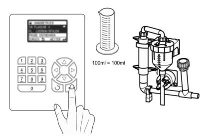
Fig. 24: Calibrate the flow-proportional dosing vessel via the System settings men
