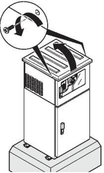
Fig. 9: Loosen the screws and remove the cover
