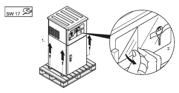
Fig. 6: Move the equipment from the transport pallet
