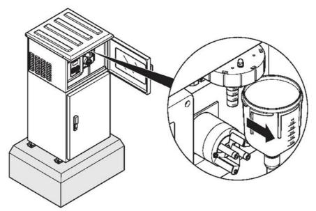
Fig. 39: Remove the dosing vessel
