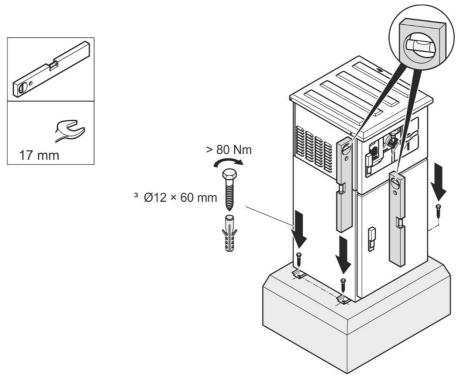
Fig. 8: Align and secure the equipment
