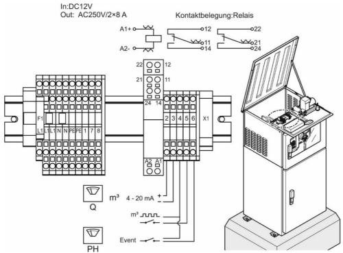
Fig. 11: Wiring diagram
