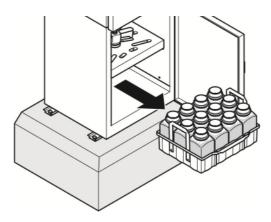
Fig. 33: Remove the full bottles
