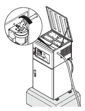
Fig. 15: Screw in the union nut
