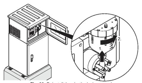
Fig. 22: Reinstall the plastic dosing vessel
