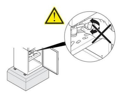
Fig. 36: NEVER rotate the distributor unit manually
