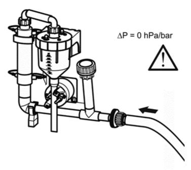
**Fig. 25:** The flow-proportional dosing vessel may only be used if there is NO counter pressure
