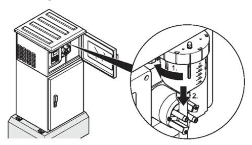
Fig. 19: Release the plastic dosing vessel
