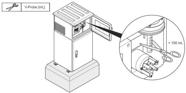
Fig. 21: Cut the dosing tube to set the sample volume (150 ml = 0.315 pt.)
